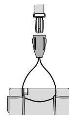
To wear the transmitter/receiver, attach the clip (5) to your clothes (e.g. belt or trouser pocket) or use the neckband: Pull the loop of the band over the clip, slide the push-button to the desired length of the band and put the band around your neck. By unlocking the snap connection (10) figure on the left), the unit is easily removed and exchanged against another one.
