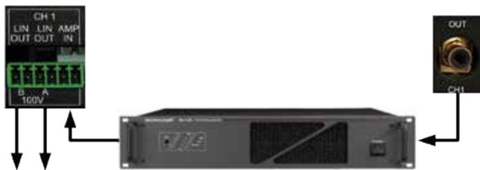
Fig. 4 Connection of a standard amplifier
